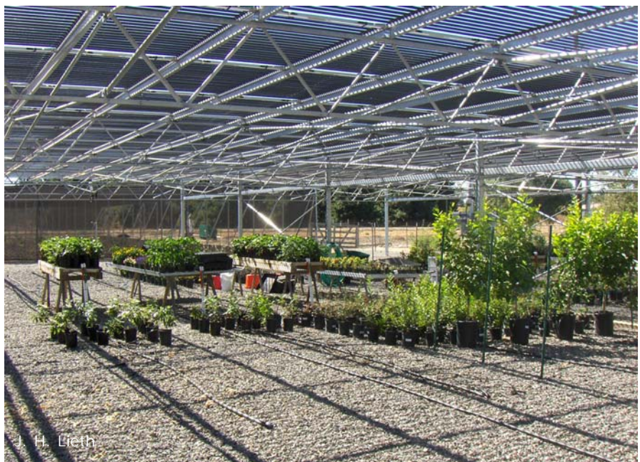
Shadehouse at UC Davis with sections constructed using conventional shade cloth or Solyndra photovoltaic panels to evaluate plant growth under these different types of shade.
