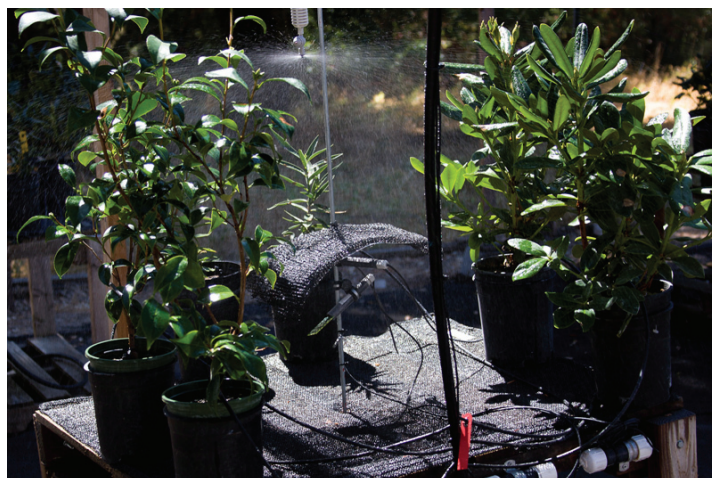
Fig. 2. To simulate fog or rain to test different leaf wetness regimes on Phytophthora ramorum sporulation, an Onset U-30 WiFi wireless datalogger with relay was used in conjunction with an Onset LW-1 Leaf Wetness sensor to control Netafim (Tel Aviv, Israel) Vibronet Mistlers (# 0354025-B). Photo by S. Tjosvold.
