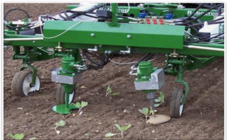
Fig. 1. The Tillet Weeder is a commercially available mechanical weed control machine that uses computer technology and a spinning blade to remove weeds. Note the disc-shaped cultivation blade with a notched cut-out to allow the blade to spin around transplanted cabbage.
