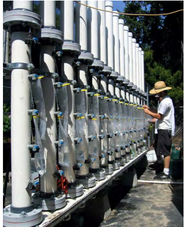
Fig. 1. Slow sand filters were constructed to study their efficacy in removing Phytophthora capsici from irrigation runoff. Graduate students Mike Harris and Corey Barnes (hidden) are collecting water samples from the filters to be examined for presence of the pathogen. Photo by Loren Oki.
