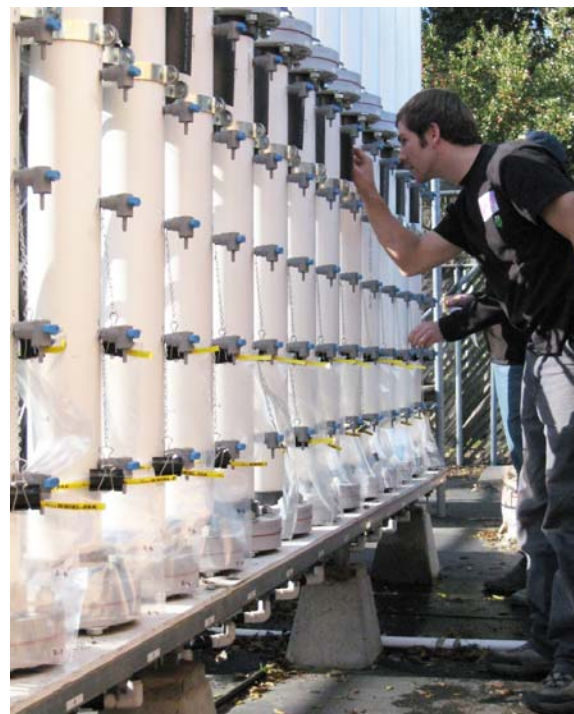
Fig. 1. Former Graduate Student Mike Harris is adjusting flow rates on slow sand filters during an experiment studying the removal of Phytophthora capsici from captured runoff water. Photo: L. Oki.
