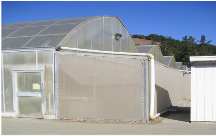
Fig. 2. One end of this greenhouse is screened to exclude pest entrance through the pad end of a fan-and-pad cooling system. Photo: J. Bethke.
